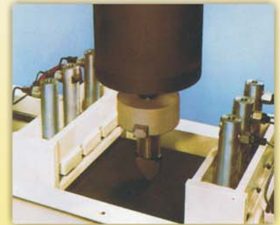
Test on resilience to impact load
